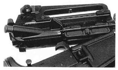
Unlatch the charging handle and pull it back, this will extract the bolt carrier group.
