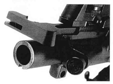
Pull the bolt carrier straight back until it is free of the charging handle and upper. Pull the charging handle back until it stops, then allow it to drop down to clear the upper receiver and remove it from the rear.
