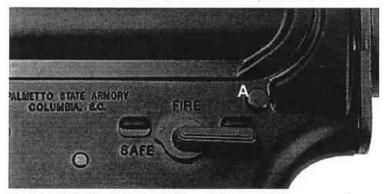
of the safety lever on the left hand side of the lower receiver.
