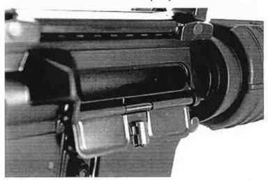
Look into the receiver through the ejection port and verify that there are no cartridges in the chamber.
