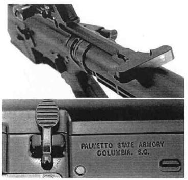
Unlock and pull the charging handle all the way out and press in on the lower portion of the bolt catch. Release charging handle. This locks the bolt in the open position.
