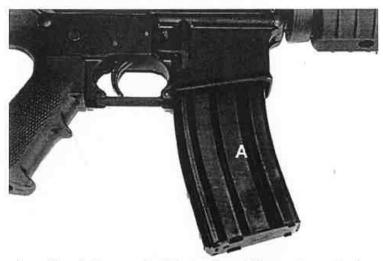
Insert loaded magazine into receiver. Give a sharp slap to the bottom of the magazine to ensure it is seated. The magazine can be inserted with the bolt open or closed. If the bolt is open, press the top of the bolt release button to close the bolt and chamber a cartridge. If the bolt is closed, pull the charging handle completely to the rear and let it go. Do not allow your hand to "ride" the charging handle, as this may cause misfeeds.
